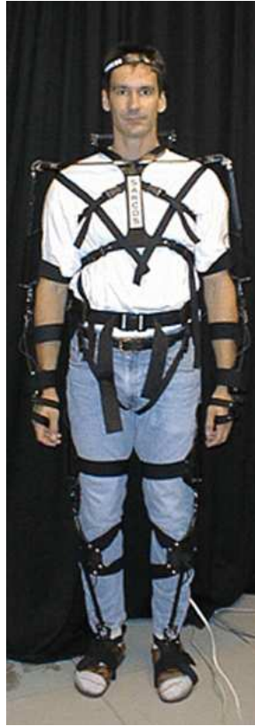
Figure 3.7: The Sarcos SenSuit is an exoskeleton that can record position data of 35 degrees of freedom of the human body at 100Hz.
